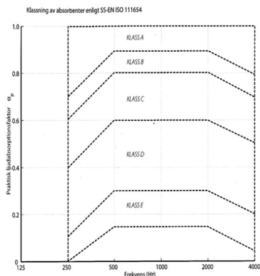
Classification of absorbents, where class A is the highest class, which corresponds to for example 100 mm mineral-wool in an under-roof.
